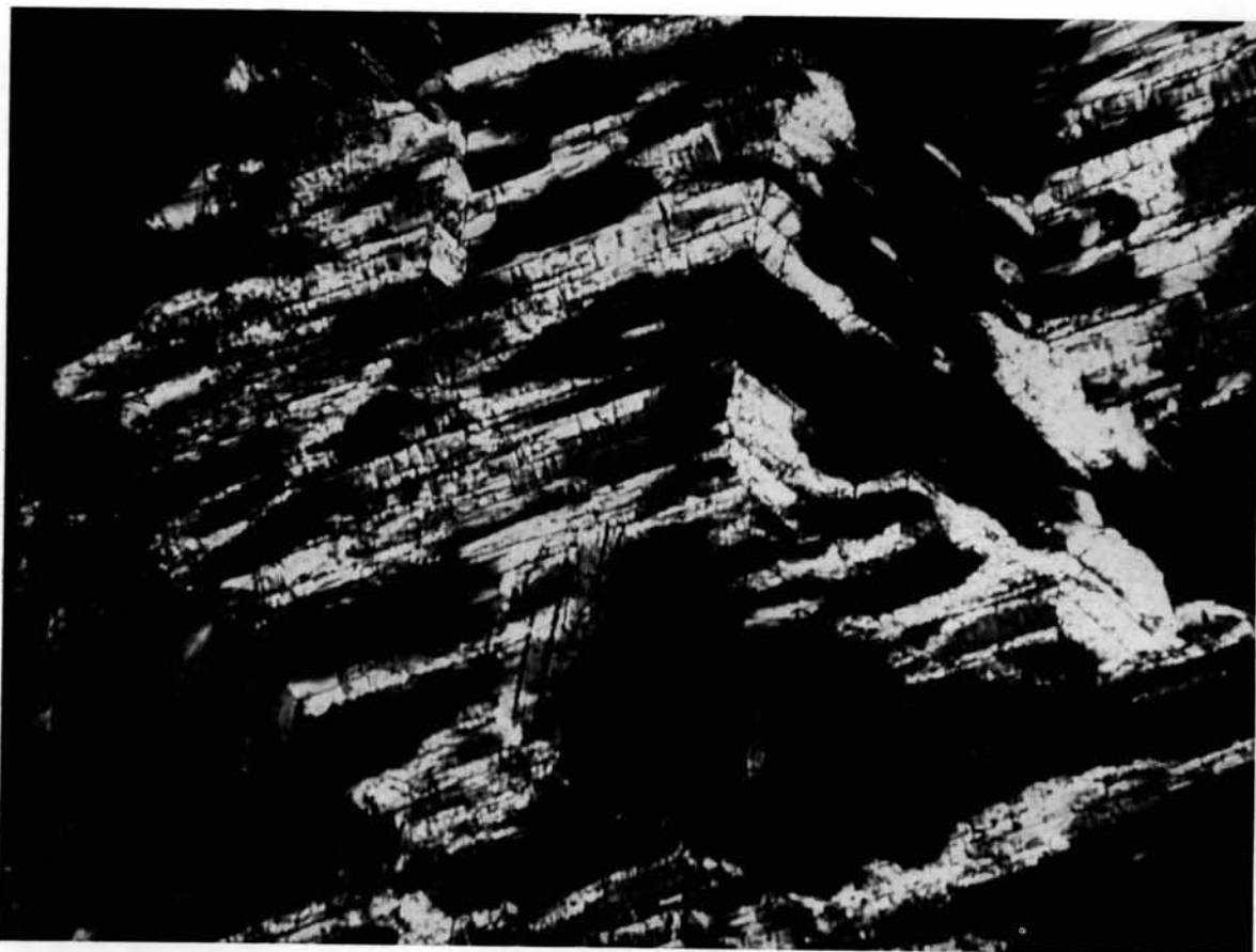
Fig. 1. Photomicrograph of a hexagonal platelet of BeO which has been heated through the transformation temperature and cooled. The domain structure which has developed has the c axes parallel to the axes intermediate between a axes of the host crystal. The crystal is about 2 mm across.
